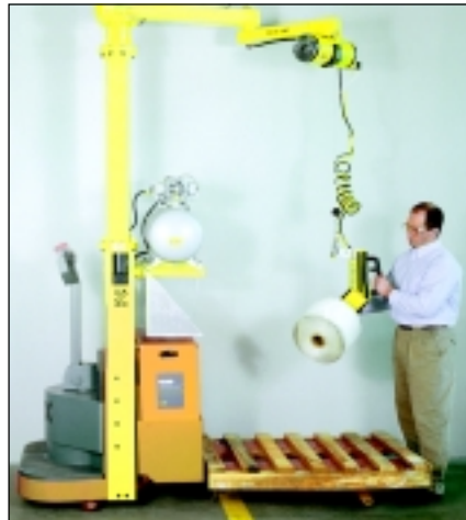
Self contained system with RAH, 720 arm, and 24 volt compressor integrated onto battery powered pallet truck. Integration to trucks, not performed by IR Zimmerman.
